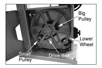
5. Reinstall the lower saw wheel with big pulley by sliding it back onto the shaft, then secure with the shaft circlip.
