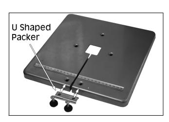
2. Guide the work table past the blade and place on the table trunnion. Position the table insert on the work table correctly.
